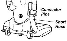
Disconnect wand from connector pipe and nozzle hose, check the wand and hose. Plug in vacuum cleaner and turn on.
